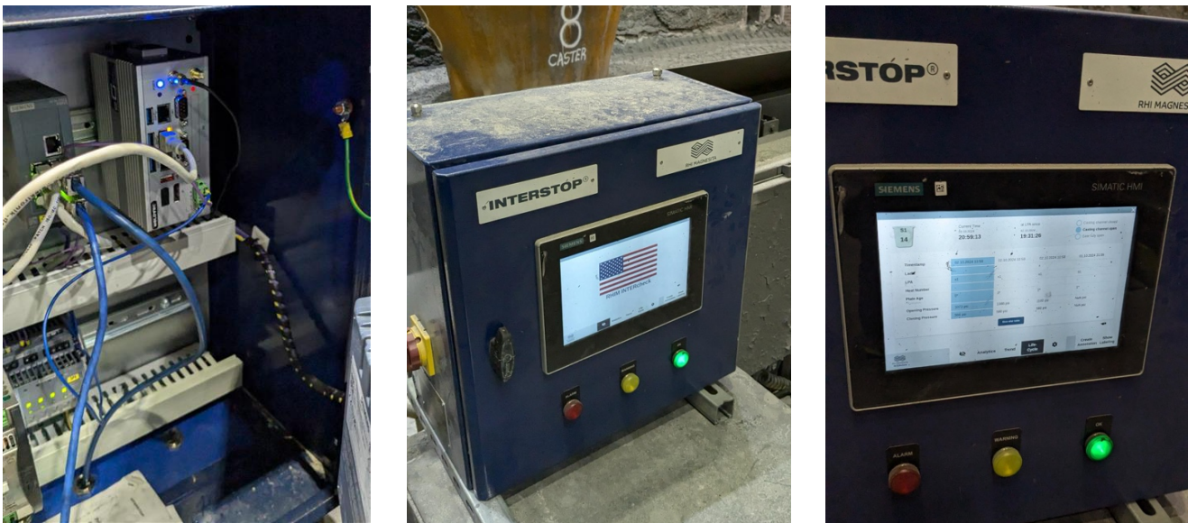
Figure 3 The platform is prepackaged on an edge computer designed for demanding industrial environments and installed at the LPA (left). Its operator-facing application (center, right) makes relevant health indicators, virtual sensors, and sensor measurements accessible via HMI directly at the LPA or via browser anywhere within the steel mill's protected network and provides a feedback interface for experts' assessment of plate health.
